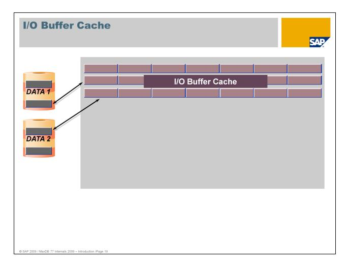
Read and write operations to the volumes are buffered in order to save time-critical disk accesses. The corresponding main memory structures are called caches. They can be dimensioned according to the user profile. The **I/O** buffer cache contains the last read- or write-accessed pages of the data volumes. It is shared by all
