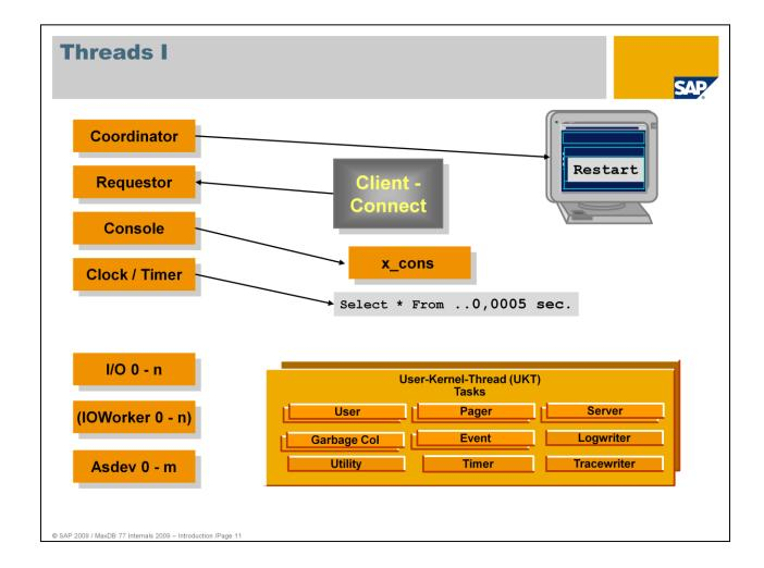
When the runtime environment is started, that is, when the database instance is started in the Admin state, first the **coordinator thread** is generated. This thread is of particular importance.
