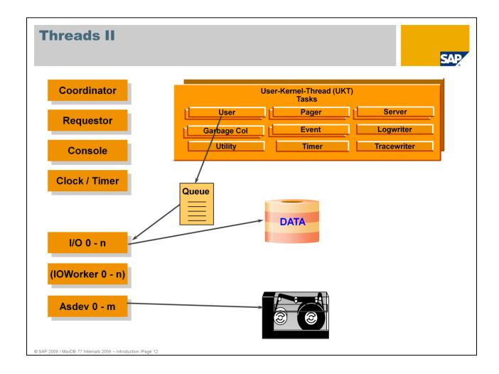
**I/O** threads are responsible for processing the write and read requests to and from data and log volumes that are requested by the corresponding tasks. MaxDB supports asynchronous I/O requests. On Windows, the asynchronous I/O of the operating system is used.
