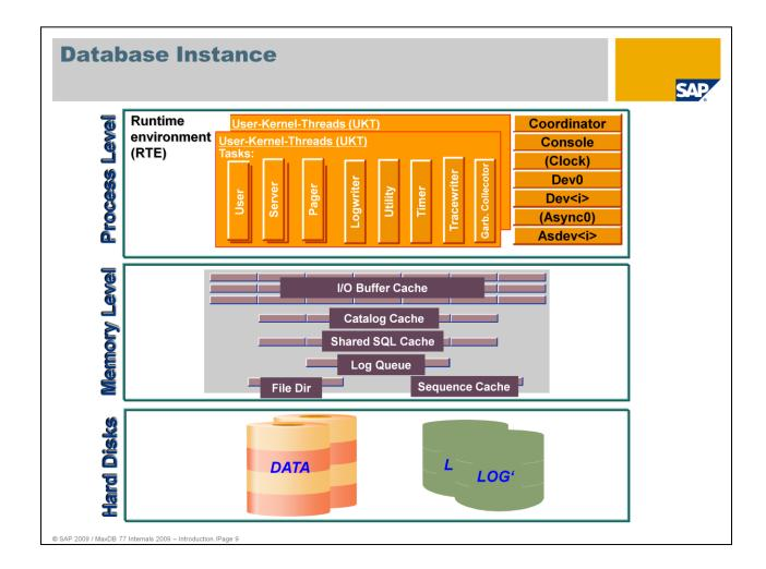
A database instance consists of the following three parts:
