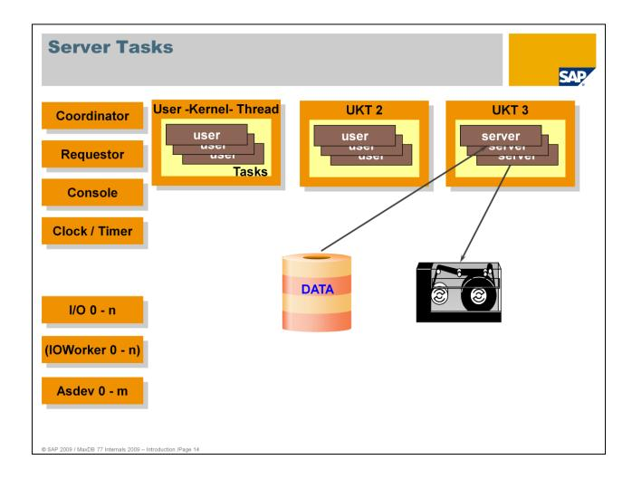
**Server tasks** are primarily used to back up data. Some server tasks read from the data volumes; others write to the backup medium.
