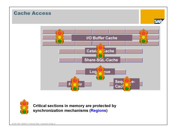
Accesses to caches can be synchronized over one or more regions. Depending on its size, the data cache is comprised of 8 to 64 segments of the same size, each of which is protected by exactly one region.
