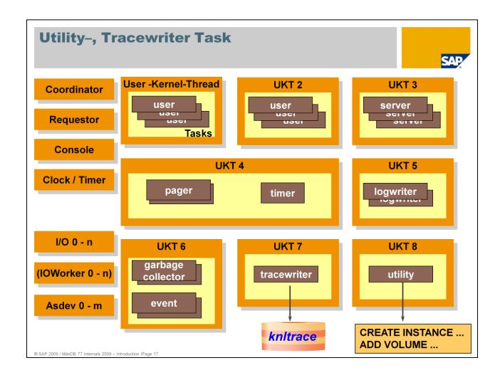
MaxDB offers the possibility of writing a special log, the database trace. The active tasks write the trace data to a buffer. If requested, the **trace writer task** writes the data from the buffer to the file knltrace.
