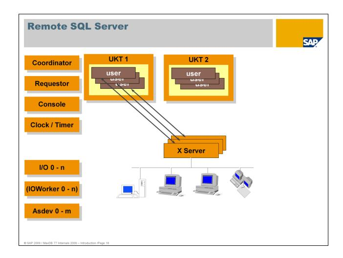
The **X-Server** is the communication server of the database system. It listens at a service port for connection requests from database applications and database tools. In the process list, this process is called **vserver**. A new vserver process is generated for every user process that logs on to the database remotely. The generating process serves the user; the new process waits for the next user logon. On Windows, an additional thread is started for the user logon.
