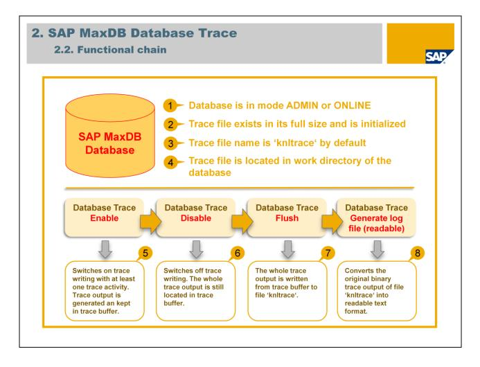
While starting the database to mode ADMIN or ONLINE a file named 'knltrace' is created in its full size. This size is calculated by the database kernel depending on other settings and cannot be changed. Size (in pages of 8KB) can be seen via parameter KernelTraceSize (1) (2).
