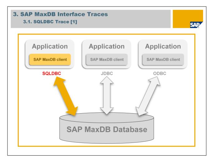
SQL Database Connectivity (SQLDBC) is a runtime library for the development of applications for MaxDB. Using SQLDBC applications can connect to MaxDB instances, execute SQL statements and process data. It consists of the runtime library libSQLDBC, the software development kit SQLDBC SDK and the tool sqldbc\_cons for tracing.
