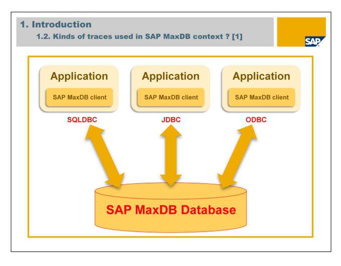
Access to a MaxDB database from application side is carried out via certain interfaces. For these interfaces corresponding MaxDB software drivers are available which are part of the MaxDB client software. Each drivers provides an own trace functionality.
