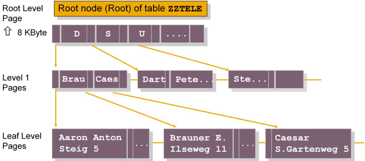
**Base data as well as index data (secondary key) is stored in B\*tree structures.**
