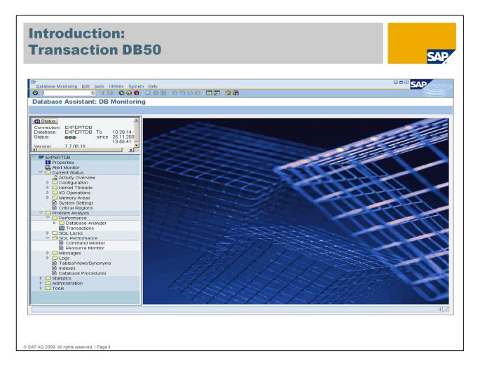
The CCMS transactions DBACockpit or DB50 are used for MaxDB database performance analysis. If you want to analyse a remote database from your SAP system you must use transaction DB59 to integrate that remote database, before you can use transaction DB50 for the analysis.
