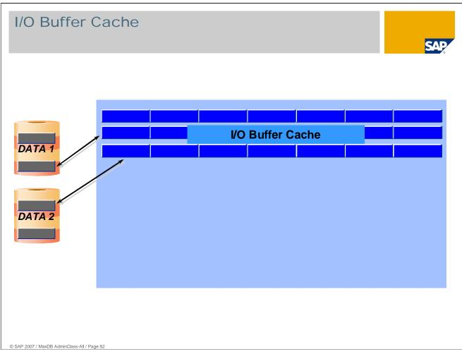
To avoid time-critical disk I/O read and write accesses to volume buffers are used. The corresponding main memory structures are named caches. Their sizes are defined by the database administrator.
