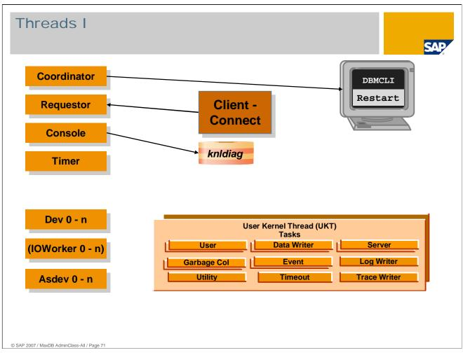
During startup of the RTE, i.e. during start of the database instance into admin state, the Coordinator Thread is created first. It has a special meaning.
