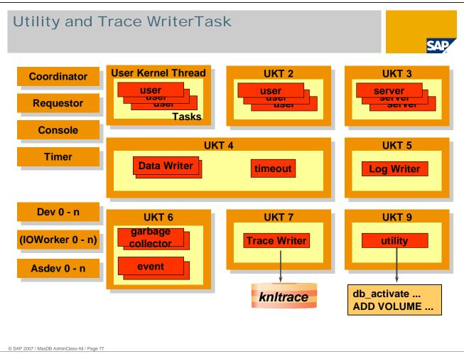
MaxDB allows to write a database trace. If this writing is enabled, the Trace Writer Task becomes active.
