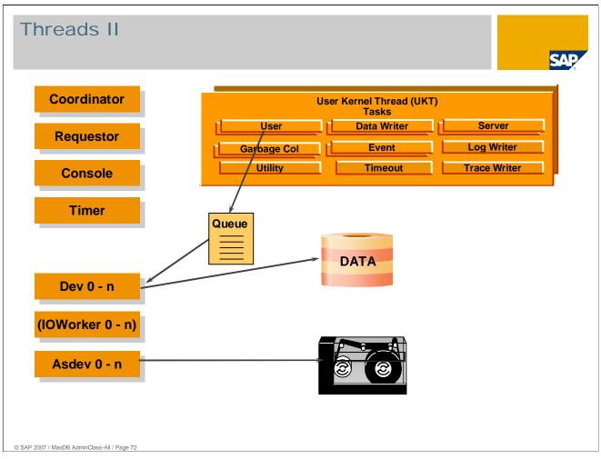
Several Dev Threads (Dev is short form of devspace, formerly used where now the word volume is used) are responsible for handling the read and write calls (sent by the corresponding tasks) to and from data and log volumes. MaxDB supports asynchronous I/O calls. With Windows NT/2000 the asynchronous I/O of the operating system is used.
