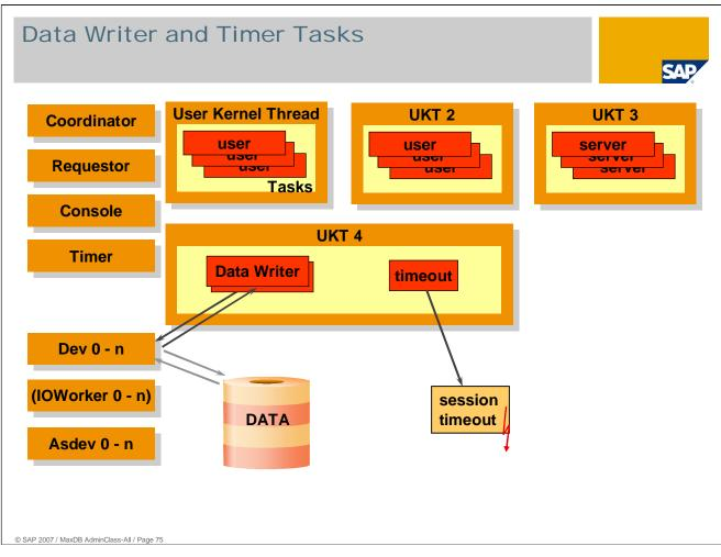
Data Writer Tasks are responsible for writing data from the I/O buffer cache onto data volumes. They become active when a SAVEPOINT has to be done. The number of Data Writer Tasks is calculated automatically by the database system. It depends mainly on the size of the I/O buffer cache and the number of data volumes.
