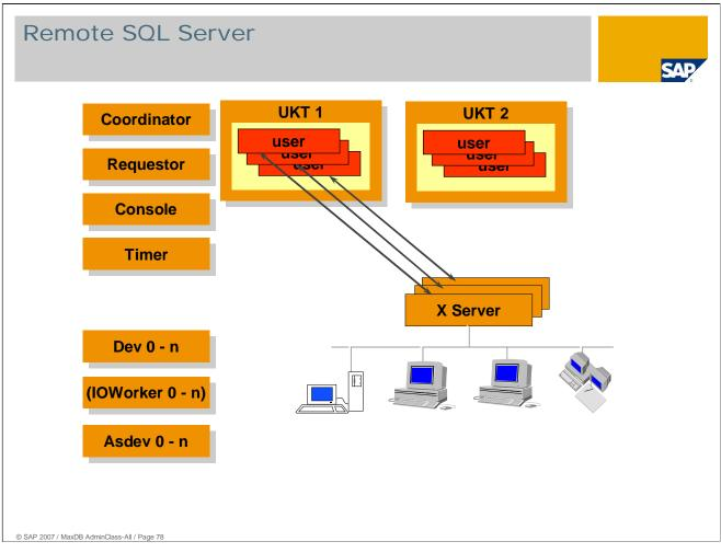
When you start the X Server on UNIX to enable remote database accesses, an additional process is created. It is named vserver. For every application process with a remote connection a new vserver process is created. The 'old' process works for the new application, the 'new' vserver process waits for the next remote connection.
