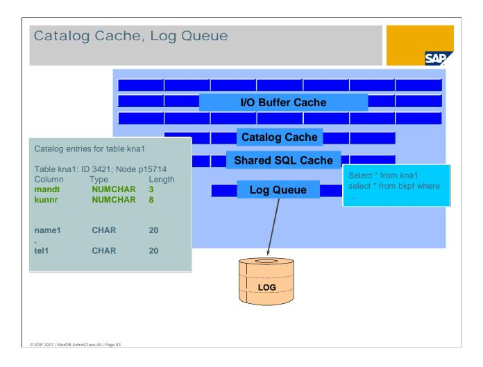
The Catalog Cache contains user specific and global catalog objects. Data displaced from the catalog cache is put into the I/O Buffer Cache. The hit rate of the Catalog Cache should exceed 85%.
