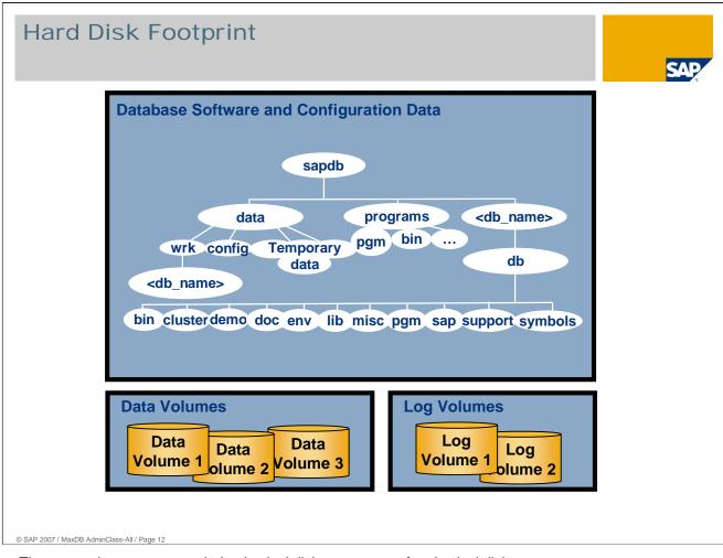
The term volume means a whole physical disk or one part of a physical disk. A database instance uses three disk areas:
