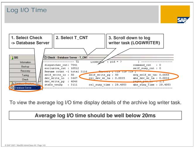
If detailed time measurement in MaxDB is enabled, the log I/O time can be obtained in DBMGUI -> Check – Database Server ->  $T_CNT$ .
