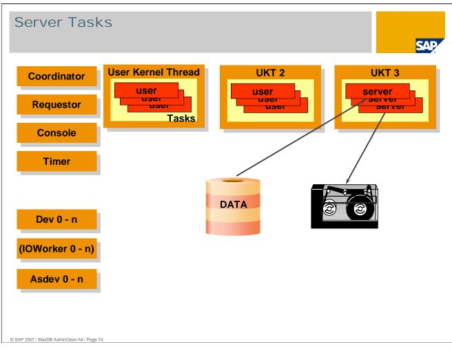
Server Tasks mainly are used for backups. Some Server Tasks read from the data volumes, others write onto the backup devices.
