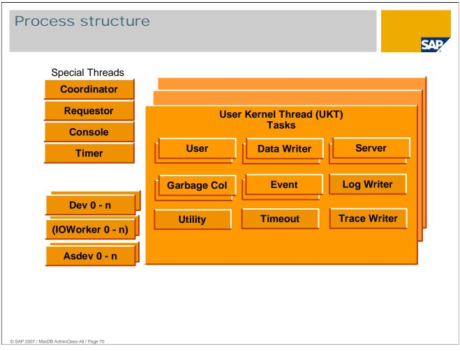
The database kernel runs as one process which is divided into threads.
