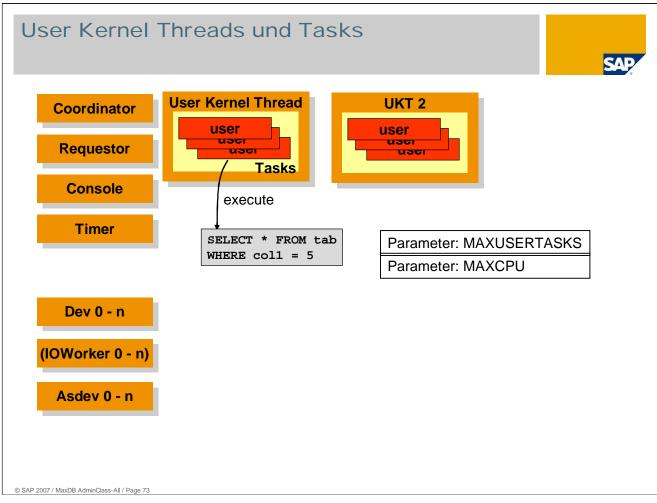
Each user respectively each application process/thread is assigned to exactly one User Task when handling the connect request. The maximum number of User Tasks available depends on the database parameter MAXUSERTASKS. This parameter therefore sets the upper limit for the number of parallel sessions for the database.
