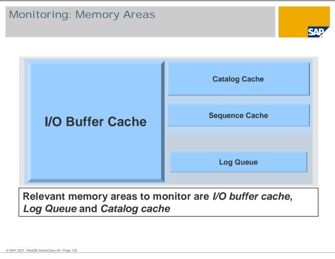
In the physical memory of the MaxDB server, MaxDB allocates the I/O buffer cache and some additional other memory areas. Generally the memory consumption of MaxDB is dominated by the I/O buffer cache.
