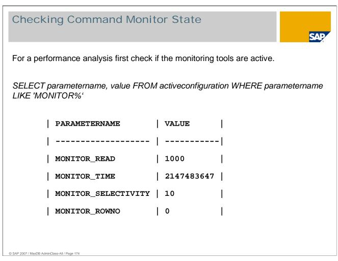
monitor\_read / monitor\_selectivity / monitor\_time: shows the values with which the command monitor was started.
