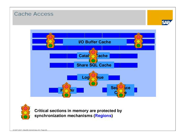
Accesses to caches can be synchronized over one or more regions. Depending on its size, the data cache is comprised of 8 to 64 segments of the same size, each of which is protected by exactly one region.
